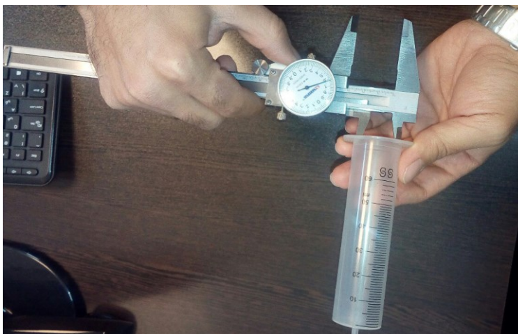
Measuring the inner diameter of syringe using a caliper
