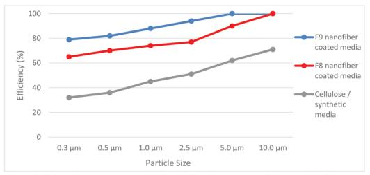
Comparison of efficiency between common air filter media and FNM's nanofiber coated air filter (F8 and F9).
